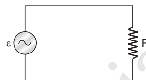
Fig. 4.1. AC voltage applied to a resistor.
