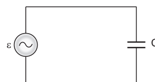
Fig. 4.5. An ac source connected to a capacitor.
